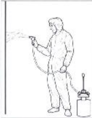
Use low-pressure spraying where possible
