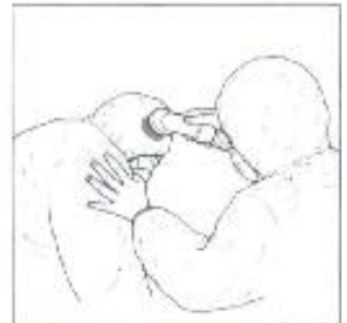
'Buddy' cleaning using a Class H vacuum cleaner
