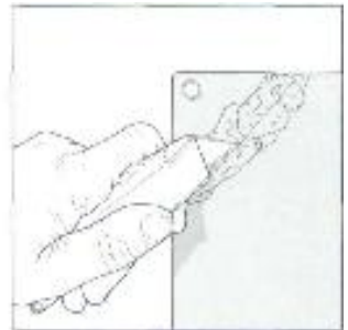
Panel with nails: If possible, remove nails with a claw and shadow vacuuming. If this is difficult without damaging the board, apply paste to one corner and make a deep score line so you can lever the corner away first
