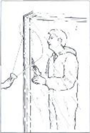
Test the enclosure for leaks with a smoke test
