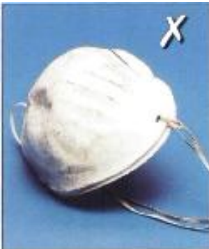
A 'dust mask' doubled up for more protection is useless. You need a respirator
