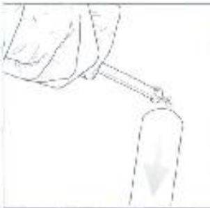
Panel with screws: Use shadow vacuuming to control dust as you remove screws
