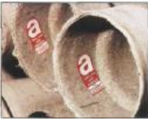
Top row: An asbestos gasket, asbestos cement pipes and an asbestos-containing fuse board Bottom row: The asbestos cement pipes are labelled, so are the tiles, but you might not know until you start to lift them. There could be sprayed limpet under the asbestos cement (AC) sheeting
